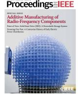
On the Cover: Our cover photo this month features a polymer-jetting-printed Eaton lens with an X-band WR-90 waveguide feed. The photo first appeared in IEEE Antennas and Wireless Propagation Letters (DOI: 10.1109/ LAWP.2015.2514181).
